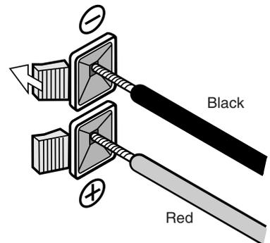
Hold down the button of the speaker terminal with your finger, insert the conductor of the connection cable, and release your finger.
