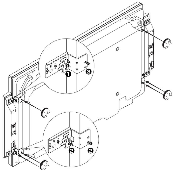
**5** Fully tighten the four partially tightened screws.
