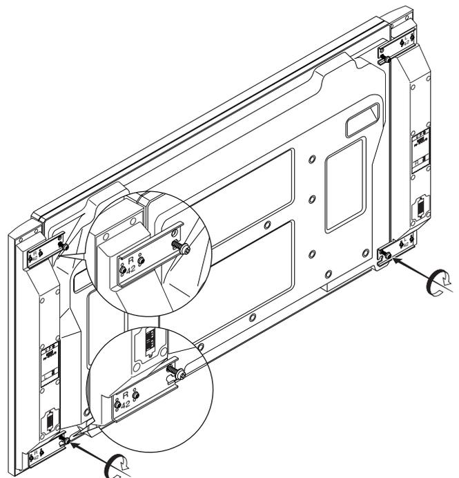
**5** Fully tighten the four partially tightened screws.
